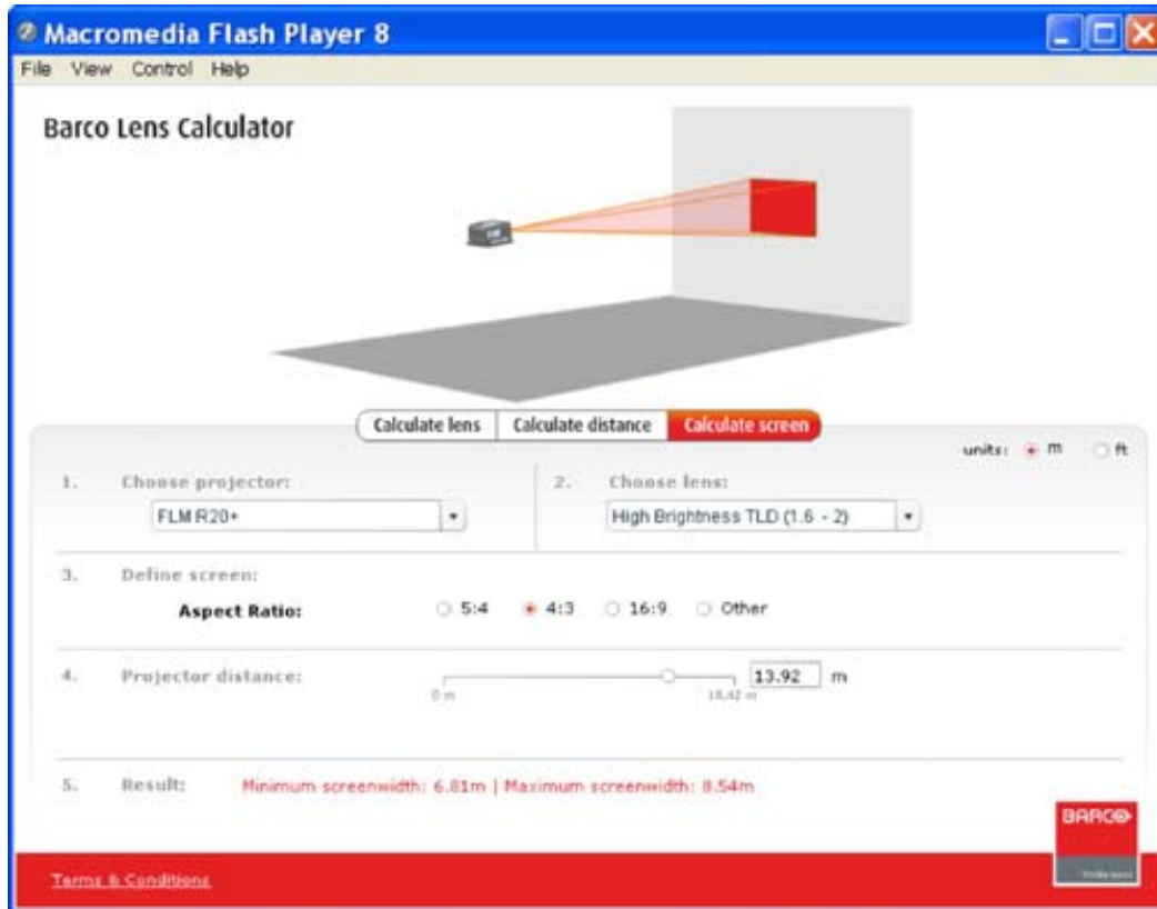
Image 16-4 Screen width calculation
