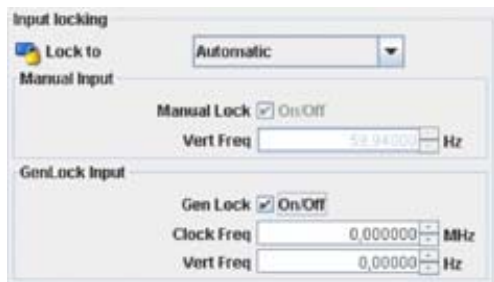
Image 6-12 Input locking, automatic or specific input options
