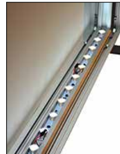
Close up view of LED lights inside lightbox
