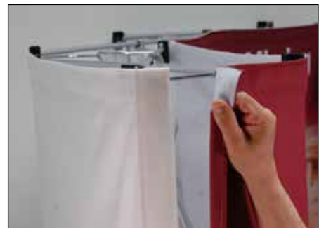
Inatallation of fabric backcover and front graphic at end cap.
