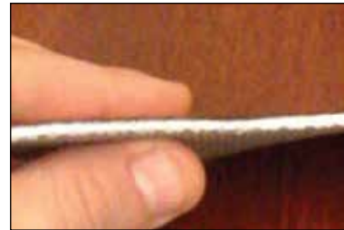
In Step carpet is 1/8" thick. This includes polyester felt and rubber backing.
