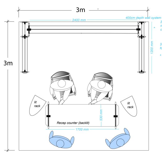
200mm depth wall system rises to height of 2400mm clamped or bolted to 400mm backwall
